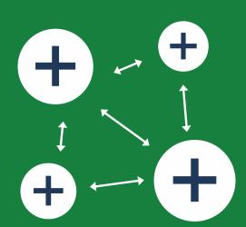
The positively charged particles repel each other like magnets, spreading evenly across the sprayed surface.
